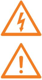
Moving chain could cause possible **SERIOUS INJURY**. DISCONNECT electric power to the operator **BEFORE** manually operating your door
