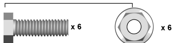
Bolt 5/16" -18 x 1" x 6 — Door arms / Mounting Opener
